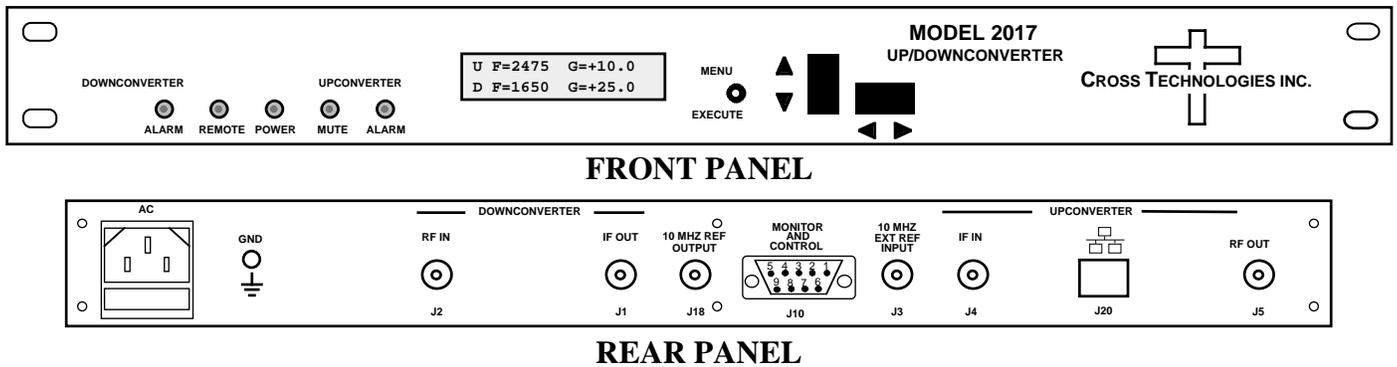
Figure 1.1 Model 2017-1625-140# Front and Rear Panels
